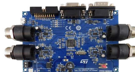
STEVAL-IDP004V1 Master board and generic RS-485/422 USB adapter
