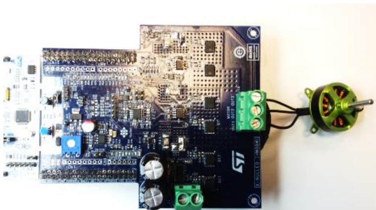
STM32 Nucleo + X-NUCLEO-IHM08M1 + LV motor
