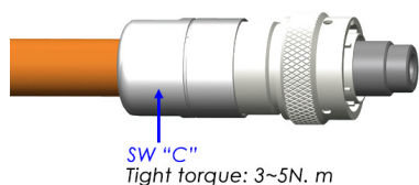
Step 9: Attach and tighten backshell as shown
