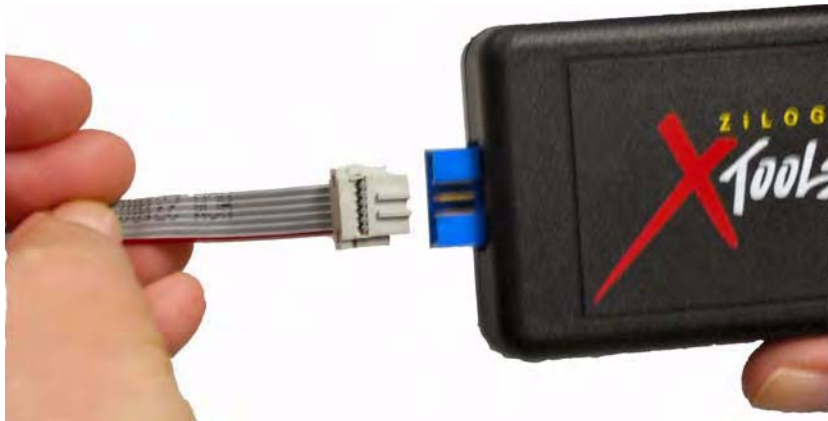
Figure 13. Connecting the 6-Circuit Ribbon Cable to the USB SmartCable
