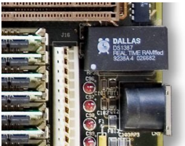
The image above shows a computer motherboard with a Real Time Clock called the
