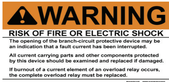
UL 508A Warning Sign
