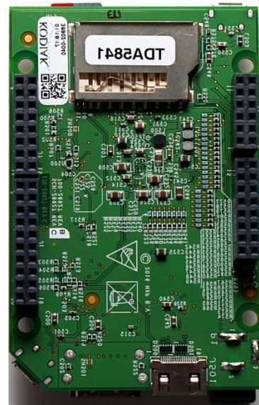
Figure 6. Back of the QWKS Board Rev C
